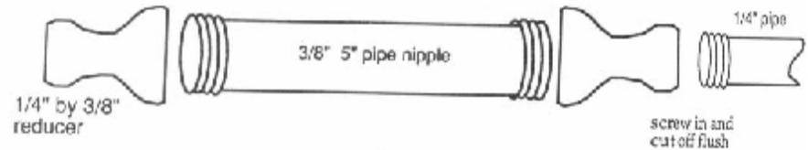
First, screw the two reducers onto the ends of the 3/8” pipe nipple and tighten them with the vise grips.
